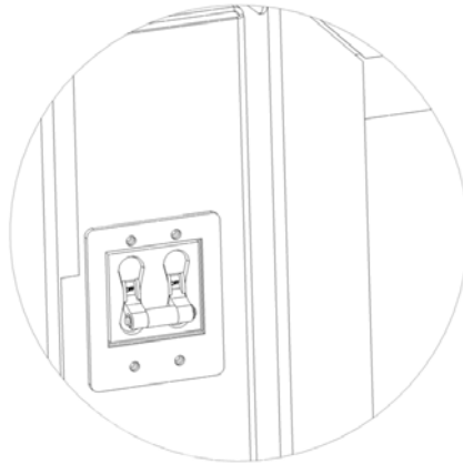
Main power breaker Figure 12
