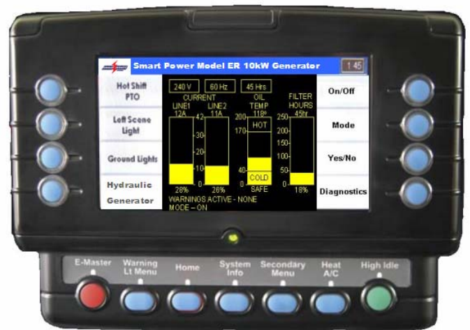
Figure 4: Generator Screen on Multiplexing Display
