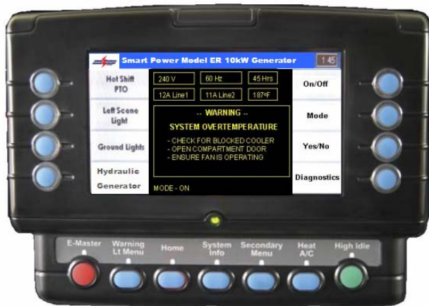
Figure 6: Generator Overtemperature Warning on Multiplexing Display
